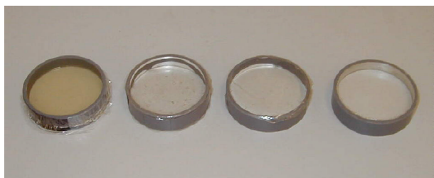
Figure4 Materials used for psychophysical experiment. Gelatine (material A), two silicon rubbers (material B,C) and acrylic polymer (material D), from left to right.
