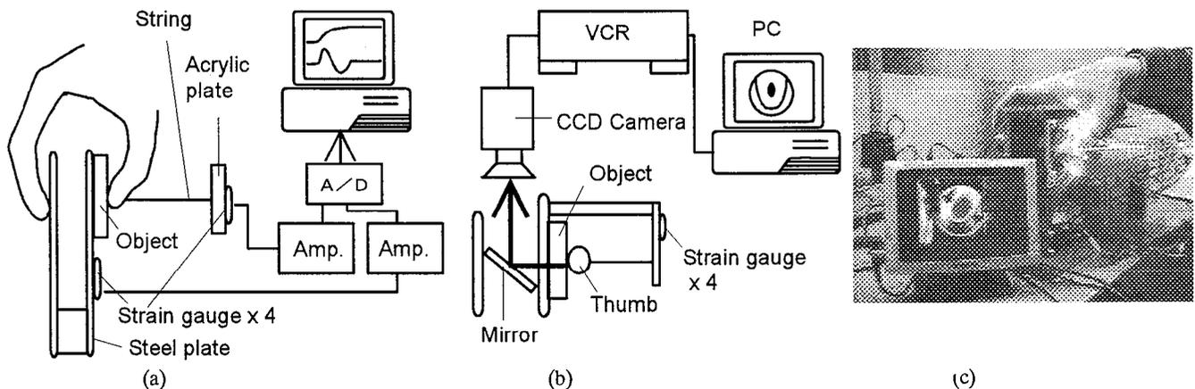
Figure 2 Experimental system to measure the pinch force, thumb displacement and contact area during pinch motion. (a) side view, (b) top view, (c) set-up.
