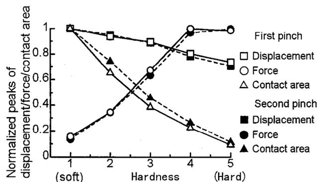
Figure4 The pinch force, object displacement and contact area during the pinch of five objects. Values are normalized by each maximal values. The object displacement was calculated from the precedently measured hardness of the object and the measured pinch force.
