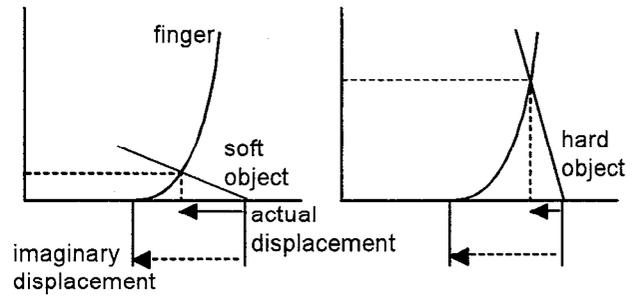
Figure7 Change of the object displacement described by the equilibrium point model.
